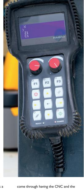
the middle is an extra that Duncan wanted because when the head is in the horizontal position you can't machine to the edge of the bed, so having a row of stops in the middle of the bed means you can work off your pods, lift it up and still have a datum to work to. You just drop down and machine in sideways. These features were requested because Duncan envisaged doing five-axis CNC work as well as nesting carcase panels."
